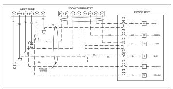
SYSTEM DIAGRAM - HEAT PUMP WITH TWO STAGE COMPRESSOR AND TWO STAGE ELECTRIC HEATER
