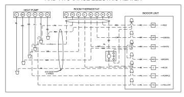
Thermostat with Low Voltage Wire to Heat Pump Unit
