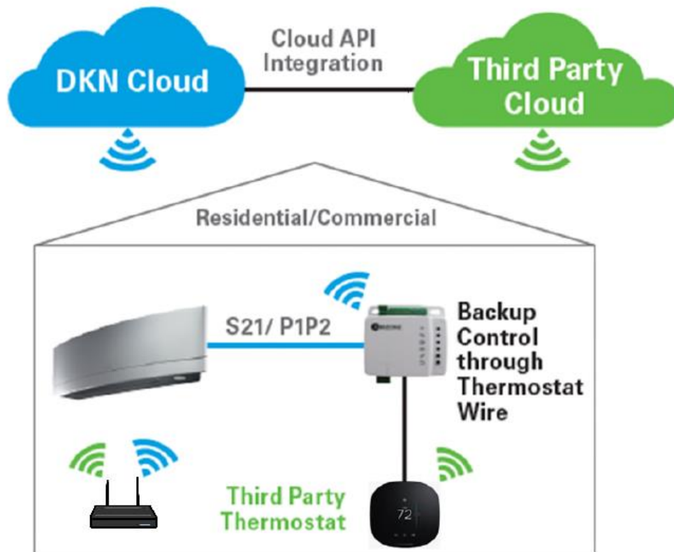
Fig 2. Cloud-to-Cloud API Connection
