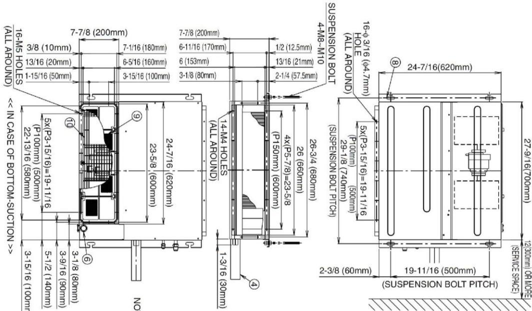
NOTE) 1. IN CASE OF BACK-SUCTION MOUNT CHAMBER COVER TO BOTTOM SIDE OF THE UNIT.
