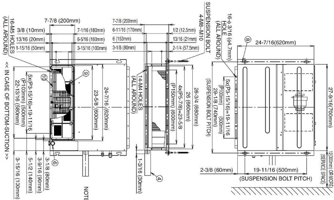
NOTE) 1. IN CASE OF BACK-SUCTION, MOUNT CHAMBER COVER TO BOTTOM SIDE OF THE UNIT.
