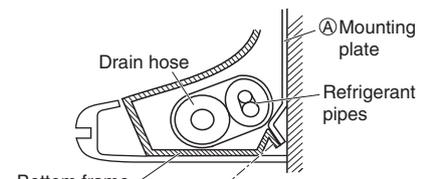
Secure the indoor unit to the (A) mounting plate with the (H) indoor unit fixing screws M4 x 1/2" (M4 x 12mm) (2 points).
