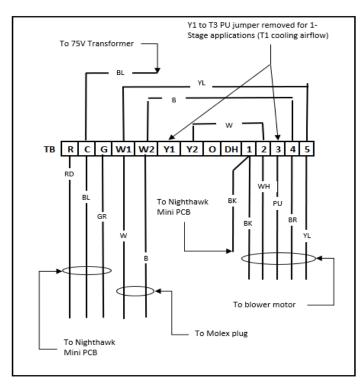
1-STAGE APPLICATIONS WIRING FIGURE 5B
