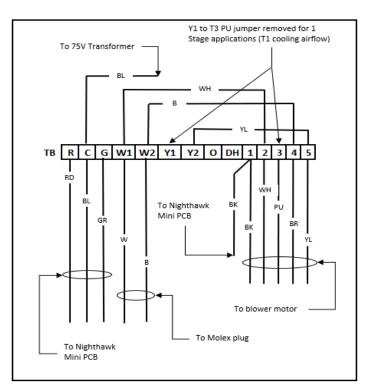
1-STAGE APPLICATIONS WIRING FIGURE 5A
