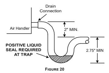
NOTE: Trapped lines are required by many local codes. In the absence of any prevailing local codes, please refer to the requirements listed in the <u>Uniform Mechanical Building Code</u>.
