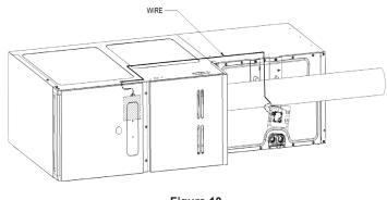
Figure 10 Horizontal Right Configuration
