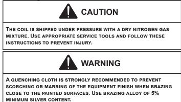
All cut ends are to be round, burr free, and cleaned. Any other condition increases the chance of a refrigerant leak. Use a pipe cutter to remove the closed end of the spun closed suction line.
