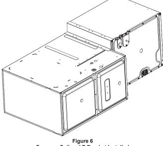
Furnace, Coil and Z-Bracket Installed
