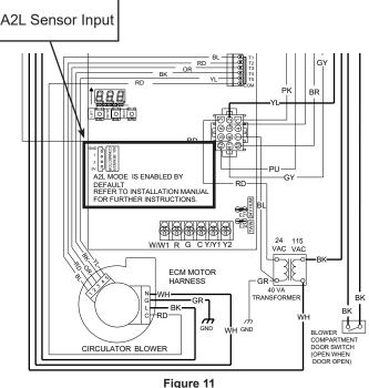
Typical Design for Refrigerant Detection Sensor Connectors
