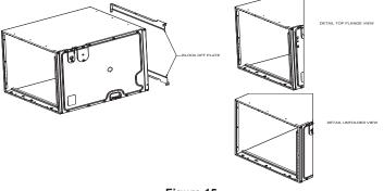
Figure 15 Block-off Plates & Duct Flange Detail
