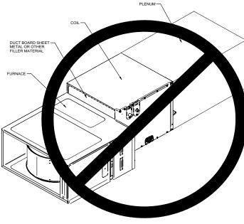
Figure 4 Incorrect Furnace, Coil and Plenum Installation
