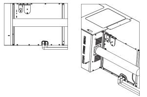
Figure 17 80% Flue Vent & Drain Port
