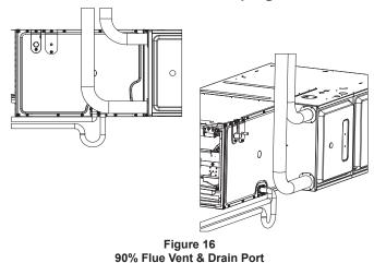
A minimum of 2.0" distance from the top of the furnace and the bottom of the coil pan is required.
