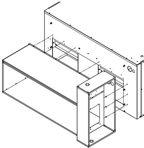
The wires from the heat kit are to be routed through the pipe nipple into the air handler electrical compartment. See the “Electrical Connection” section of this manual for wiring details.
