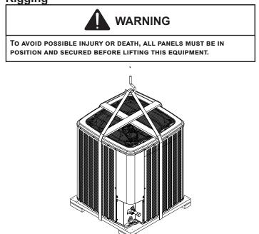
Use field-supplied spreader bars when lifting the unit to minimize the possibility of lifting cable/straps damage. To protect the cabinet louvers, use protective material such as plywood behind the cable/straps. Arrange the straps to form a central suspension point. **NOTE:** When raising and setting the unit, observe all safety rules. Remove shipping skid and all protection and lifting material after the unit is in place.
