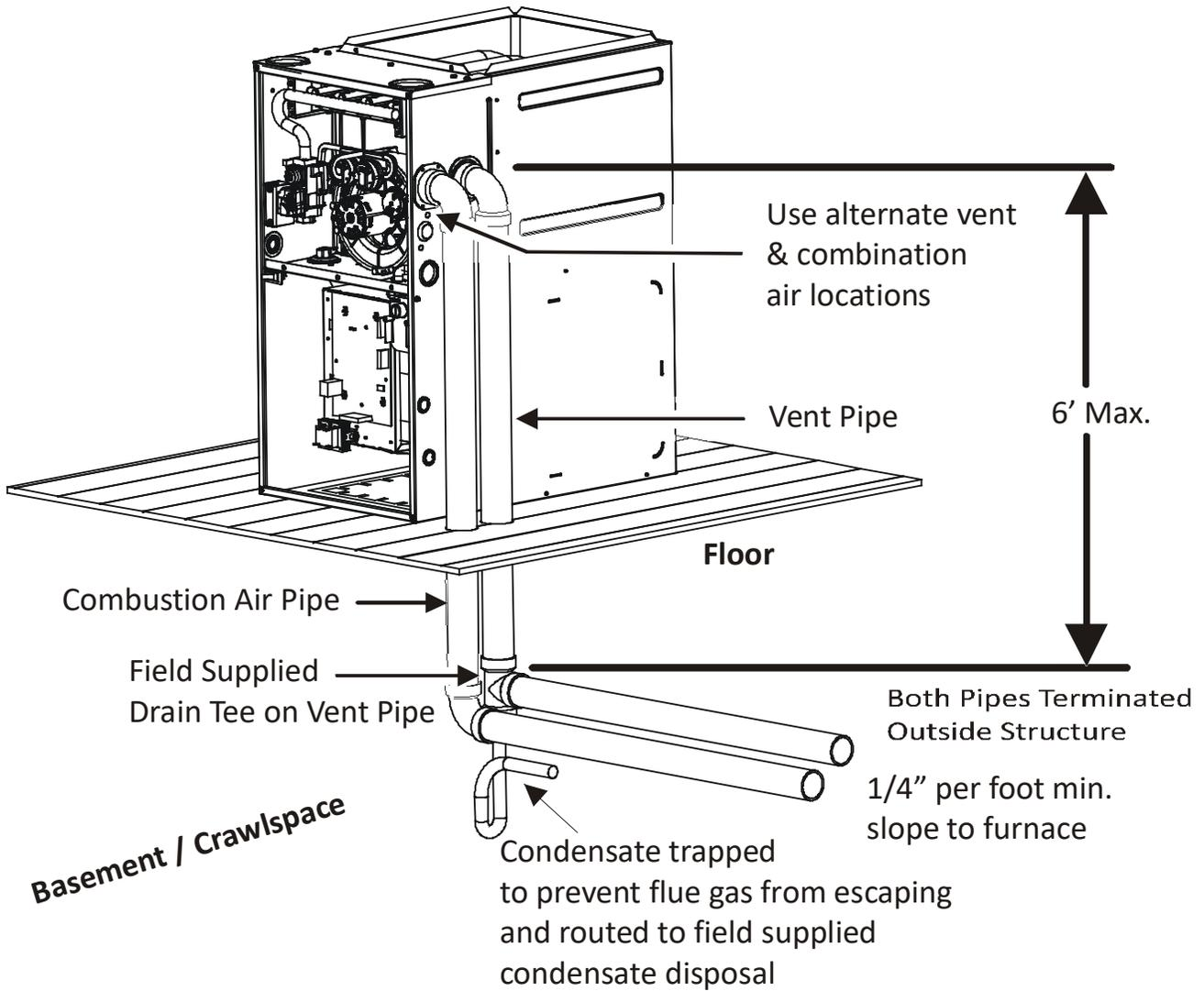
*All piping and fittings must be joined per material manufacturers specifications to prevent separation and flue gas leaks.*
