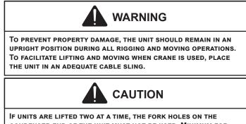
IF UNITS ARE LIFTED TWO AT A TIME, THE FORK HOLES ON THE CONDENSER END OF THE UNIT MUST NOT BE USED. MINIMUM FOR LENGTH IS 42" TO PREVENT DAMAGE TO THE UNIT; HOWEVER, 48" IS RECOMMENDED.
