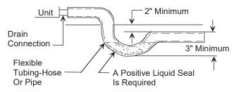
FIGURE 7: CONDENSATE DRAIN TRAP PLUMBING
