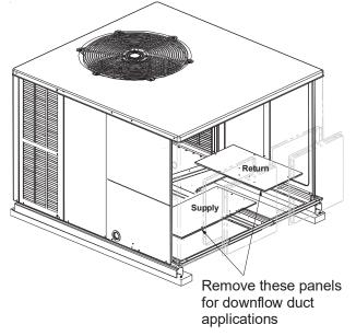
FIGURE 5B: DOWNFLOW DUCT COVER INSTALLATION
