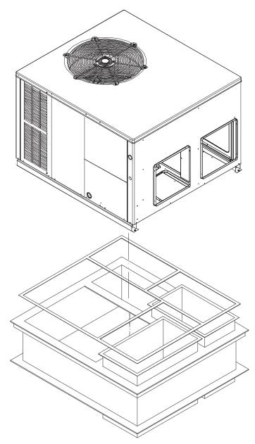
FIGURE 3: ROOFCURB INSTALLATION
