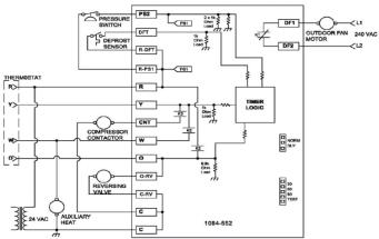
FIGURE 12: DEFROST CONTROL WIRING SCHEMATIC
