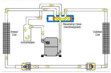
FIGURE 10: HEAT PUMP HEATING SCHEMATIC
