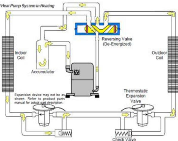
For Heat Pump units, the expansion devices are Fixed Thermal Expansion Devices (TXV) and perform the same function on the heating cycle as on the cooling cycle. The Fixed TXV also act as check valves to allow for the reverse of refrigerant flow.
