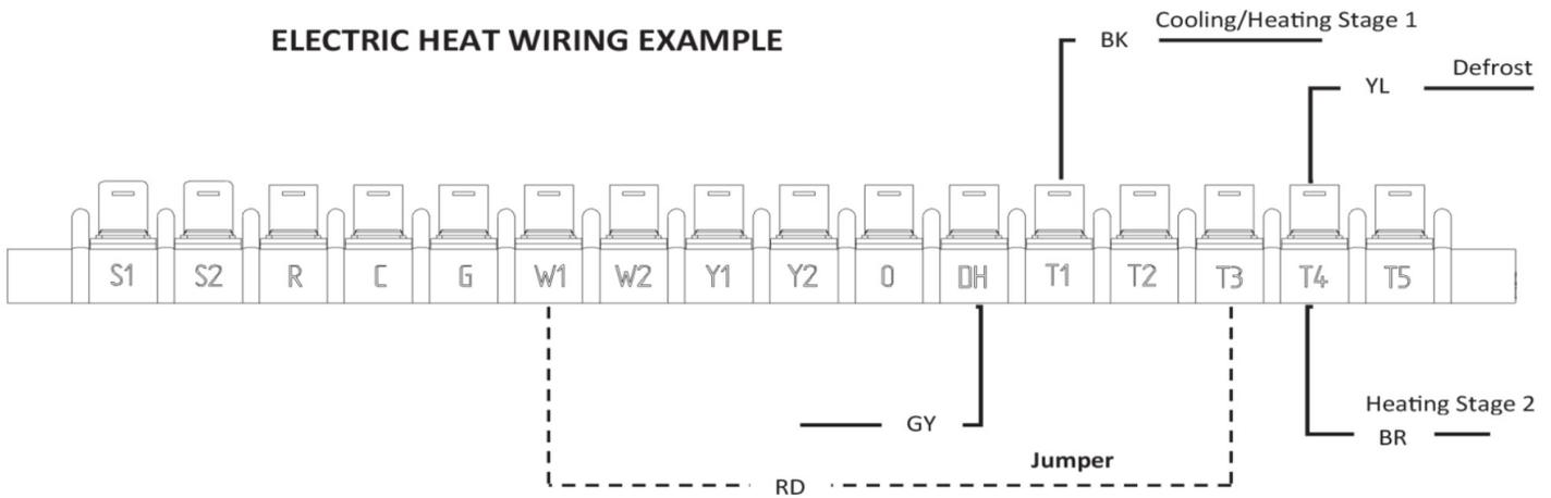
\*Move BROWN (BR) wire from TB1-T2 to T3, T4 or T5 to change blower speed during heating stage 2 operation.
