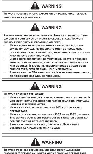
DISPOSABLE) SERVICE CYLINDERS WHEN REMOVING REFRIGERANT FROM A SYSTEM.
