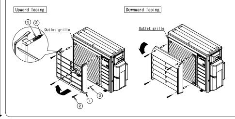
Appearance of the air direction adjustment grille after installation (when installed with the louvers facing up)
