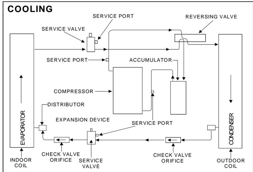
If the out door ambient is low and the unit operates properly on the heating cycle, you may check the pressure cutout operation by blocking off the indoor return air until the unit trips.
