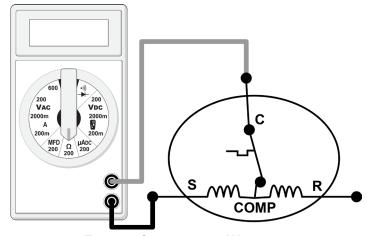
**TESTING COMPRESSOR WINDINGS**
