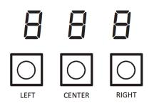
The air handler includes three on-board push buttons allowing users to navigate indoor and outdoor system menus. The Right and Left buttons allow the user to scroll through the main menus and to then scroll through available options within specific menus. The Center button is used to enter into a main menu and to then permanently select options within those menus.
