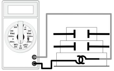
**TESTING COIL CIRCUIT**
