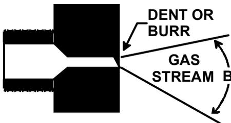
A dent or burr will cause severe deflection of the gas stream.
