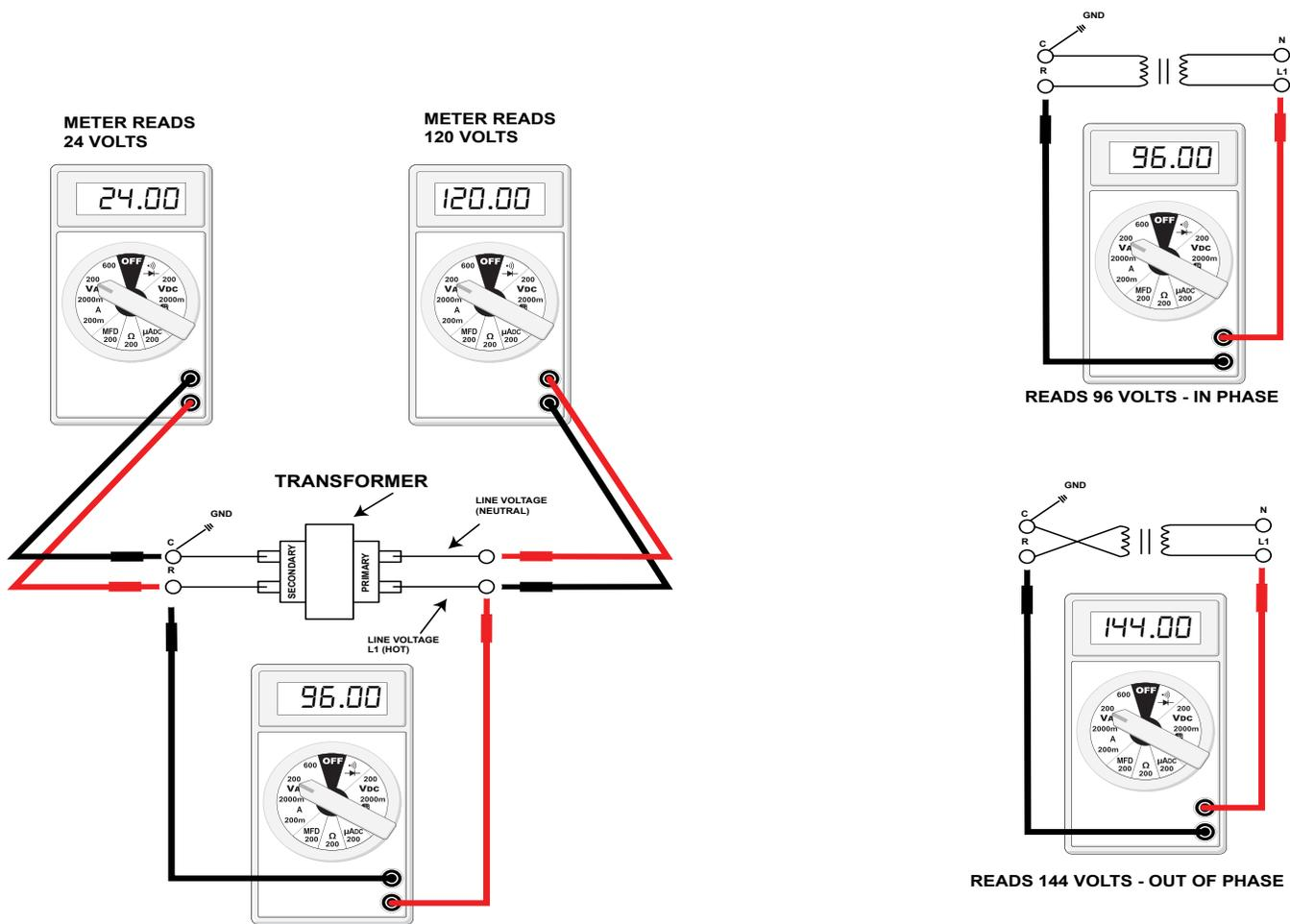
If meter reads approximately 96 volts - the primary to secondary are in phase - if reads approximately 144 volts out of phase - reverse low voltage wires.
