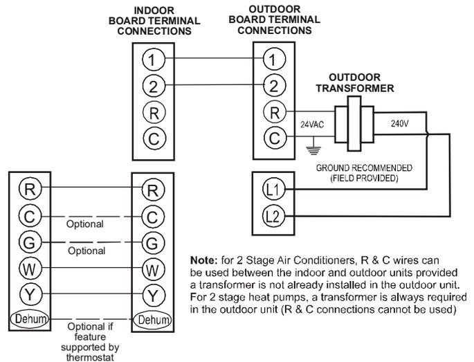
**Note:** for 2 Stage Air Conditioners, R & C wires can be used between the indoor and outdoor units provided a transformer is not already installed in the outdoor unit. For 2 stage heat pumps, a transformer is always required in the outdoor unit (R & C connections cannot be used)
