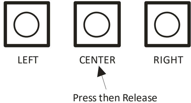
8. Press and Release the Center Button again. The 45 being displayed will stop flashing. To then complete the selection process and make 45 the official fan only setting Press and Release the Center Button for the last time. This final step will jump the user back to the main menu list and FSd will be displayed again.
