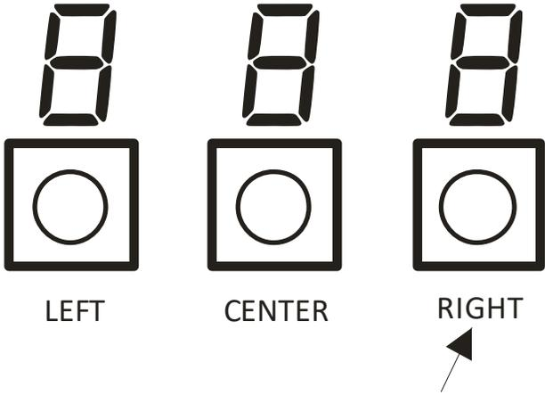
2. Press and release the Right Button (this will cycle through the menus in one direction. Pressing the Left Button would cycle through the menus in the opposite direction. For this example, the right button will be used).
