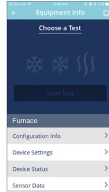
This furnace is Bluetooth ready and functions with a custom phone application designed to improve the setup / diagnostic experience of the installing contractor.
