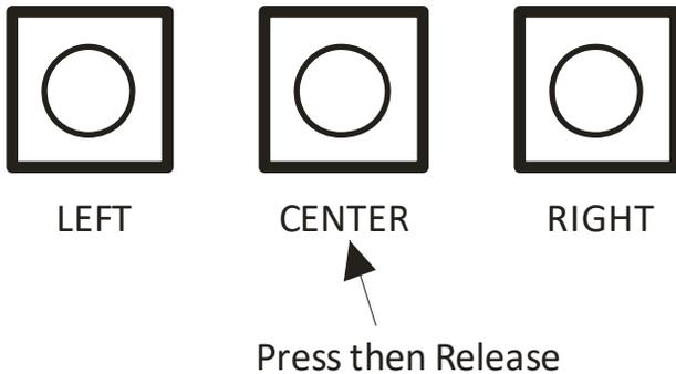
4. Press and release the Center Button. The center button is used to enter menus and make selections within menus.
