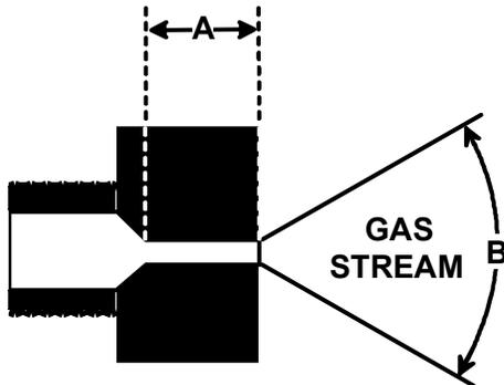
The length of Dimension "A" determines the angle of Gas Stream "B".
