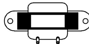
**IMPORTANT: IF THE INDUCTOR FAILS, THERE WILL BE NO MOTOR OPERATION SINCE THIS IS THE "LINE" POWER SUPPLY, BLACK WIRE, FROM THE INTEGRATED IGNITION CONTROL TO THE MOTOR. TO DETERMINE IF THE INDUCTOR IS AT FAULT, YOU CAN BYPASS BY THE INDUCTOR BY DISCONNECTING THE BLACK WIRE FROM THE INDUCTOR AND CONNECTING IT DIRECTLY TO THE MOTOR. IF THE MOTOR OPERATES THEN THE INDUCTOR WILL NEED TO BE REPLACED.**
