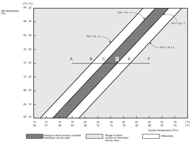
Assuming the set temperature in the figure above is 24°C (75°F), and the suction temperature has changed from 18°C (64°F) to 30°C (86°F) (A → F):
