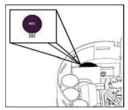
6. Inspect the large capacitors inside the control/end bell. Replace the control/end bell if any of the capacitors are bulging or swollen.
