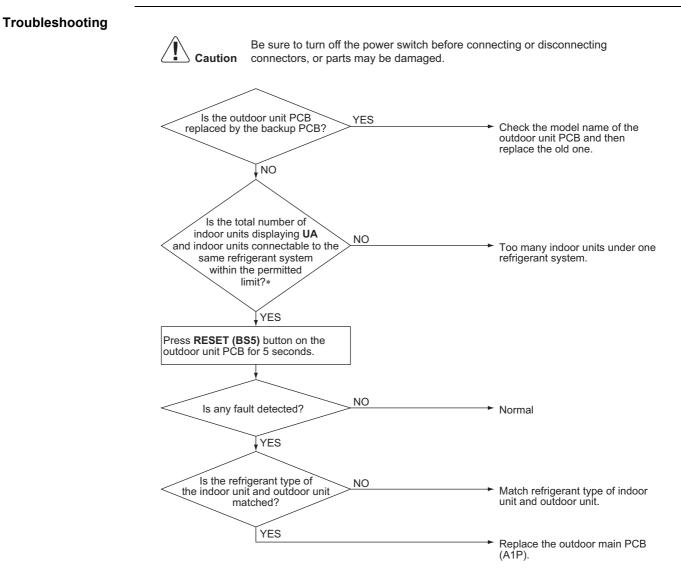
\* The number of indoor units that may be connected to an individual outdoor unit system is determined by the model of the outdoor unit.
