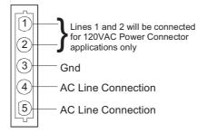
5. Measure voltage between pins 4 and 3. Voltage should be approximately half of the voltage measured in step 4.
