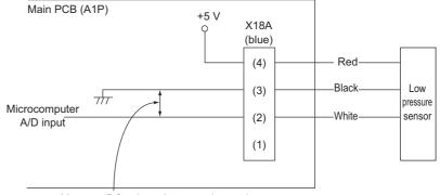
Measure DC voltage between these wires.
