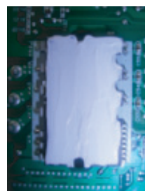
OK : Evenly applied silicon grease.
